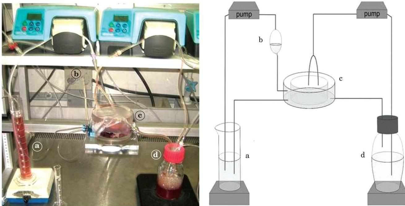
The fetal reservoir (a) is located on the left-hand side and the maternal reservoir (d) on the right-hand side, each on top of a magnetic stirring device. The fetal in-flow tubing contains a bubble trap (b), above which are the two peristaltic pumps. In the centre of the set-up is the perfusion chamber (c). The whole system is located in a heated flow bench that keeps it at a temperature of 37°C.
