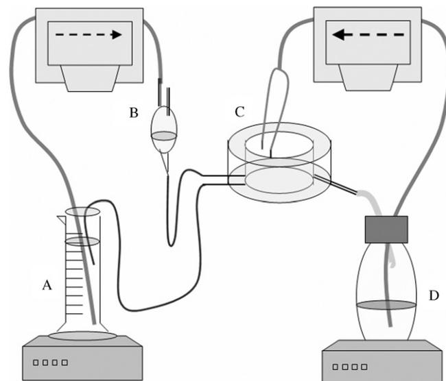
**Fig. 1.** The placental perfusion setup in Copenhagen. The fetal reservoir (A) is on the left hand side and the maternal (D) on the right hand side and placed on magnetic stirring devices. The fetal inflow tubing contains a bubble trap (B). Above are the peristaltic pumps and in the middle is the perfusion chamber (C) depicted without the placental lobule. The whole system is located in a heated flow bench which keeps it at 37 °C.
