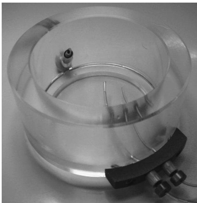
**Fig. 2.** Perfusion chamber used by Knudsen et al. [3]. The finally applied chamber with a solid surface and a gravity exit of maternal perfusion media in the wall of the perfusion chamber.
